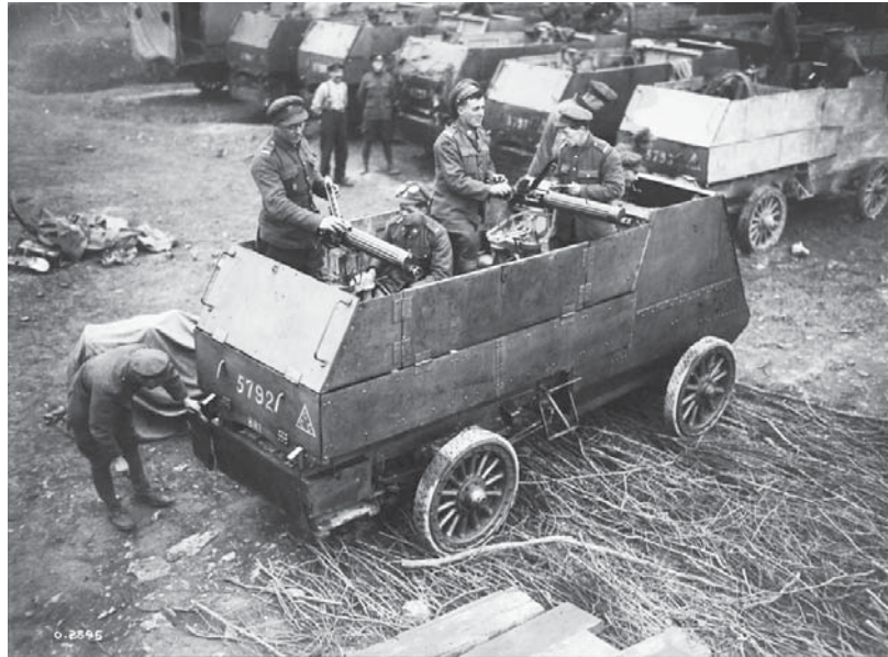
Fig. 1. Armoured Autocar, 1st Canadian Motor Machine Gun Brigade, Citadel, Arras, 1918. This is one of eight such vehicles that Raymond Brutinel took overseas in October 1914. Note the Vickers machine guns, which the unit received to replace their originally issued Colts, in August 1916. LAC Mikan3395368
